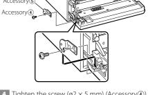
4 Tighten the screw ( $\emptyset$ 2 × 5 mm) (Accessorv(4)) and bracket (Accessory(6)) in the hole shown on the diagram.
